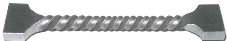
fig. 4: HSD steel probe with TWIP-effect twisted about 10\pi . The resulting deformation is up to 100%
